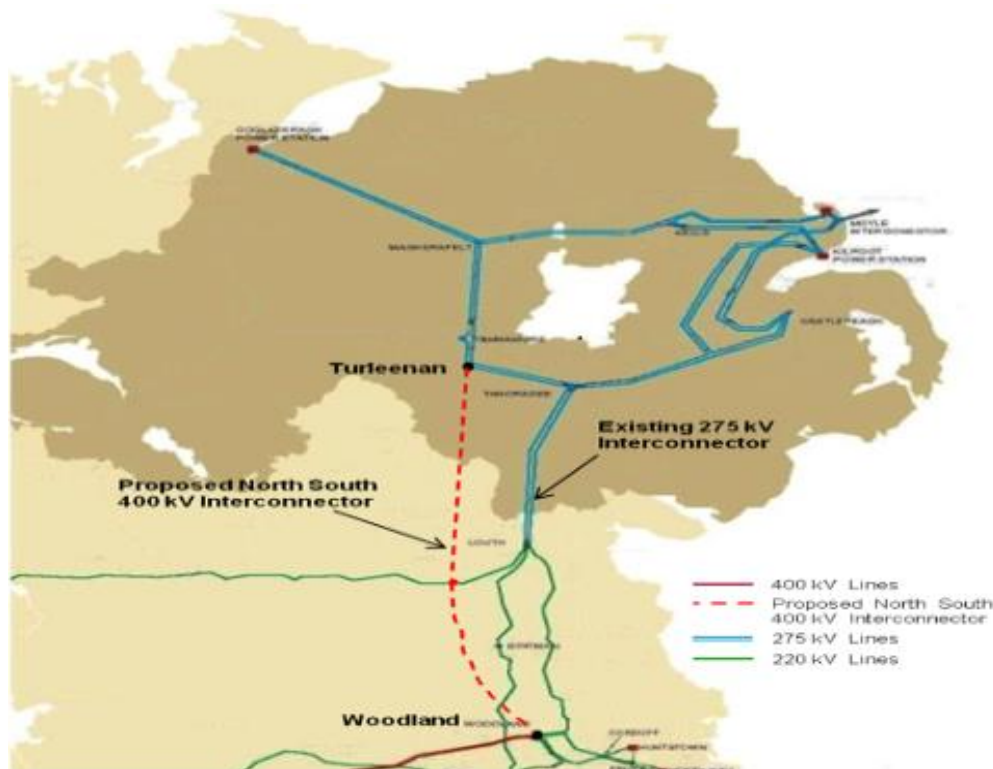
Figure 5: North-South 400 kV Interconnection Map
